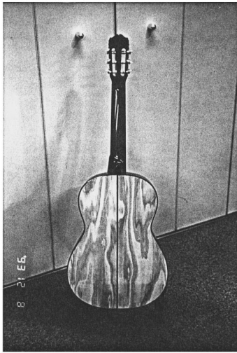
FIG. 10. Guitar with a veneer-laminated back plate.
